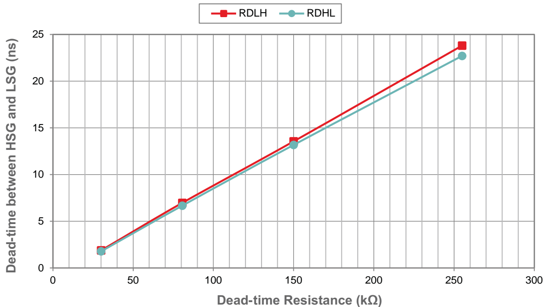
Figure 6 • Dead Time vs Dead time Resistor
