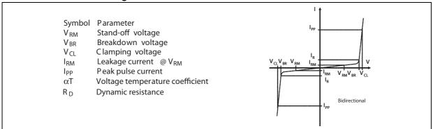
Figure 2. Pulse definition for electrical characteristics
