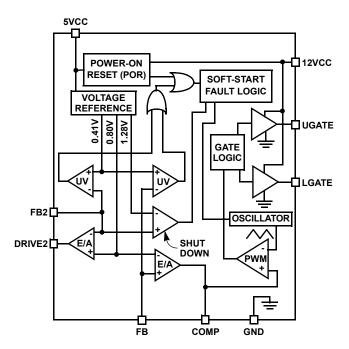
FIGURE 2. ISL6529 BASIC BLOCK DIAGRAM
