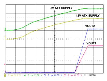
FIGURE 3. SOFT-START WAVEFORMS
