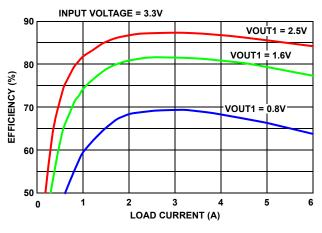
FIGURE 7. EFFICIENCY vs LOAD CURRENT FOR 3 OUTPUT VOLTAGES
